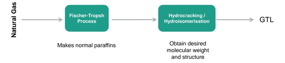
Process is well controlled and can be adjusted to make different molecular structures with predictable properties
