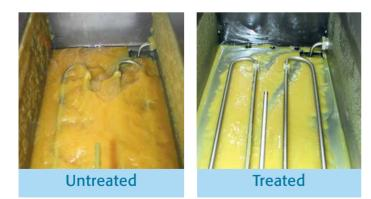
Figure 1: Infineum in-house wax settling test bench test demonstrating the effect of crude oil treated with Infineum additive solutions.
