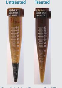
Figure 3: Asphaltene Dispersancy Test, ADT
