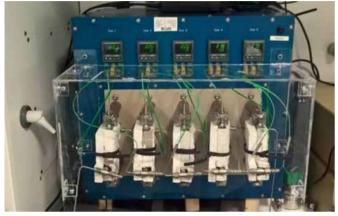
Figure 5: Image shows the Infineum 5-rod thermal deposition rig.
